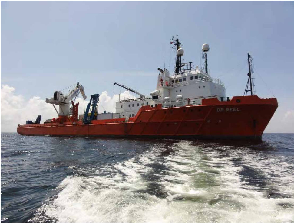
Figure 57 – Subsea cable repair vessel (DP Reel)
